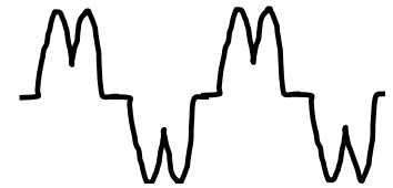
Typical current through LPF output stage
